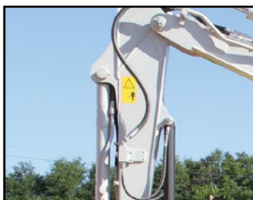
Auxiliary Hydraulic Lines
